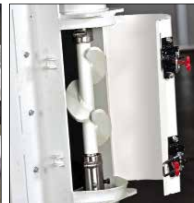
Removable hopper bottom offers easy cleanout and maintenance
